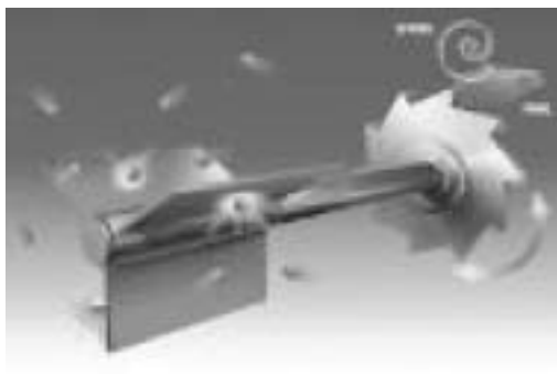
Figure 1: The Pawl machine is consisting of a vane and a wheel that can only turn in one sense of rotation. The vane is in a thermal bath of gas molecules at equilibrium. The whole device is considered to be reduced to microscopic size so gas molecules can randomly bombard the vane to produce motion.
